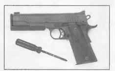
the thumb safety, which, after many thousands of rounds, was sometimes dropping the hammer. The front strap was checkered to 20 LPI and hex-head grip screws were installed for cosmetic reasons. A pair of Kim Ahrends cocobolo tactical grips were also installed.
